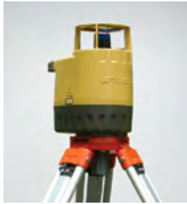
Laser Transmission Equipment
